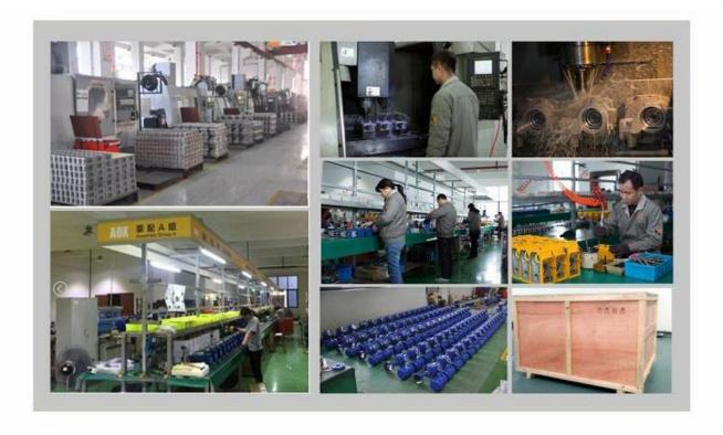
Our company has been engaged in the manufacture of electric actuators for more than 20 years. It has mature manufacturing technology and perfect production equipment, with an annual production capacity of 60,000 electric actuators. The main processing equipment includes machining center, CNC lathe, CNC milling machine, CNC drilling machine, CNC drilling
